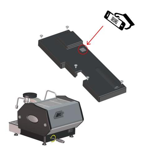
Stick one of the QR-codes on the electronic box and stick the other one in the inside of the black frame (alongside the water tank).
